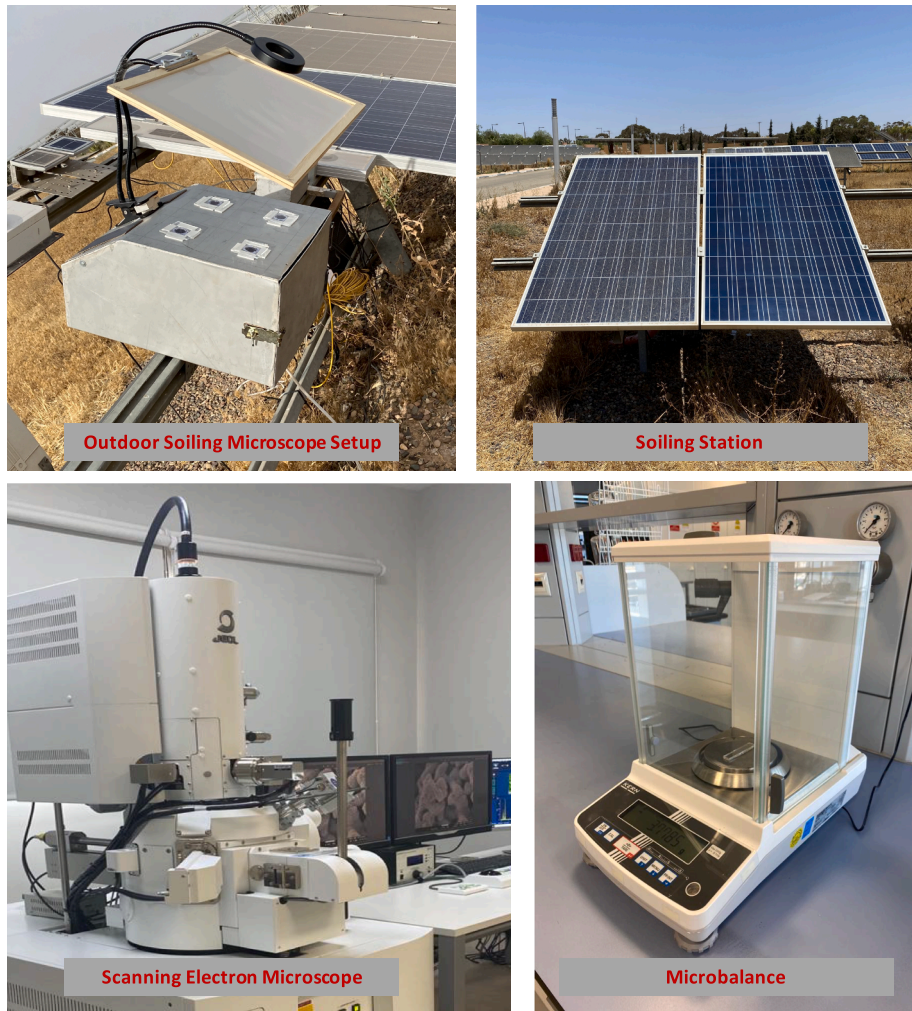
Fig. 1. Outdoor soiling assessment experimental setup and laboratory measuring equipment: (Top left) Outdoor Soiling Microscope; (Top right) Soiling measuring station; (Bottom left) JSM-7900F field emission Scanning Electron Microscope used for the characterization of dust shape, morphology, and size; and (Bottom right) Microbalance utilized for the measurement of accumulated dust mass.
